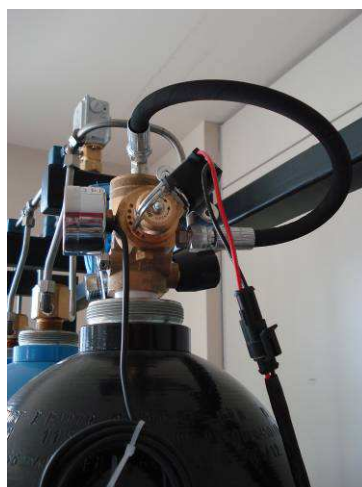
Fig. 7.2 Installation of the solenoid
