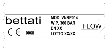
Fig. 2.24 Mark on the non-return valve for CE approval of the component
