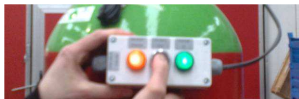
Fig. 5.11 Tester device lamps are turned on: gas is discharging.
