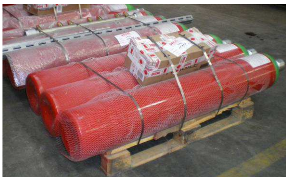
Fig. 1.3a Cylinders located on pallets (horizontal position)
