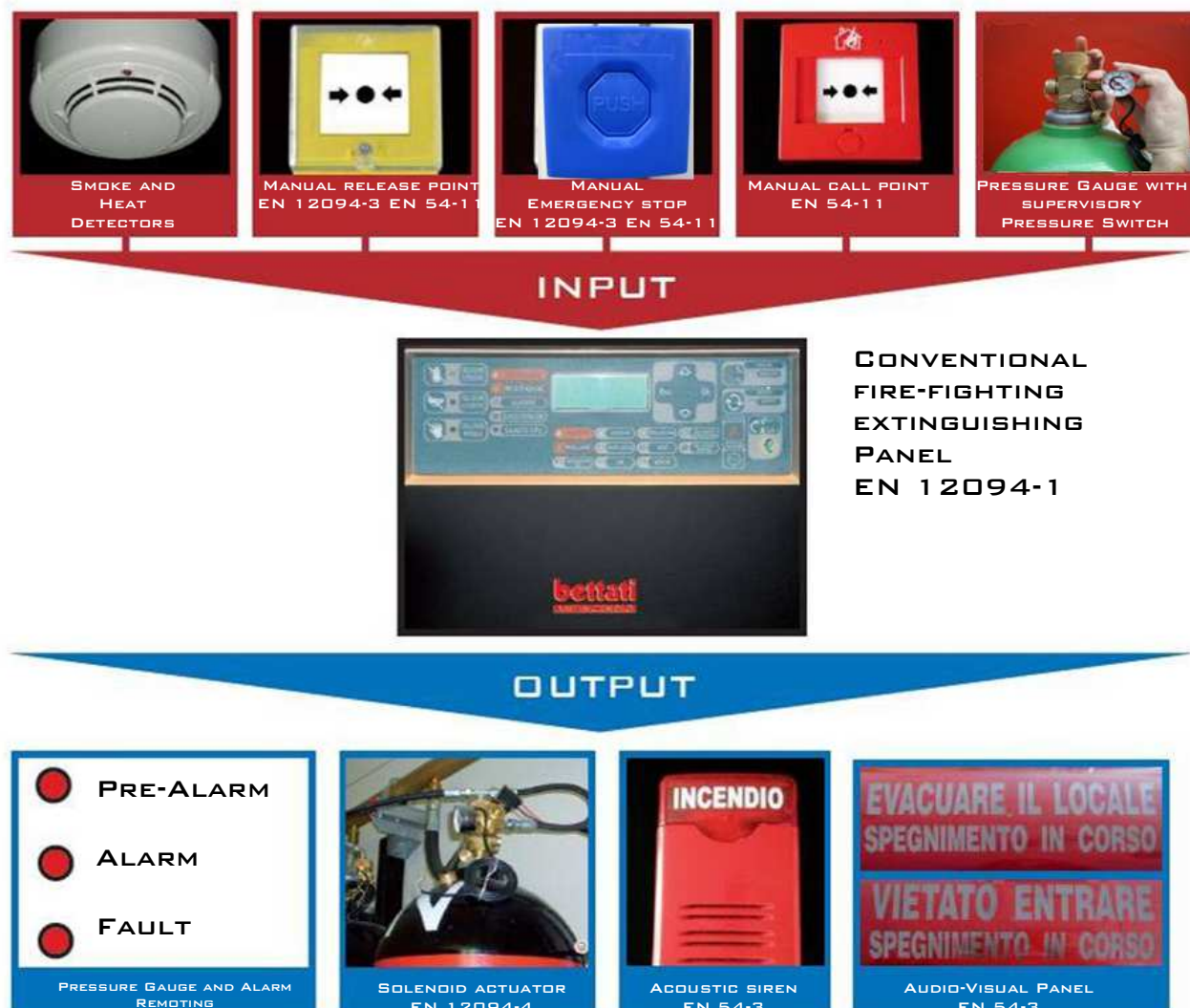
Fig.1.2 List of components of the detection system
