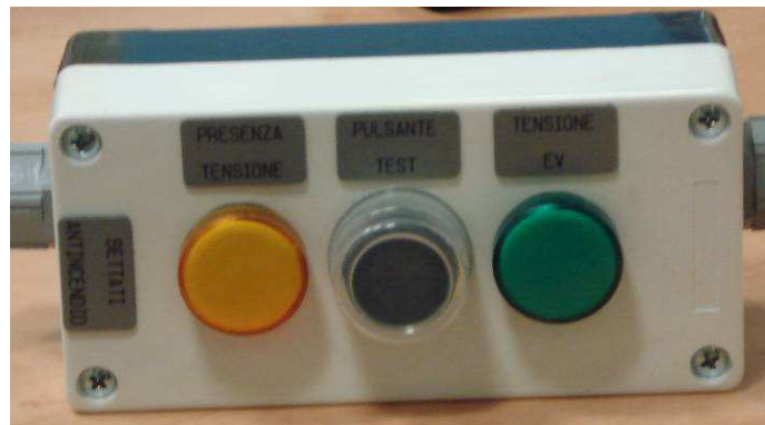
Fig. 5.8 Device for functional test of the fire-fighting system (tester device)
