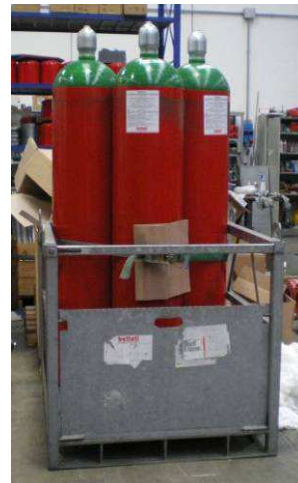
Fig. 1.3b Cylinders placed in a container (vertical position)
