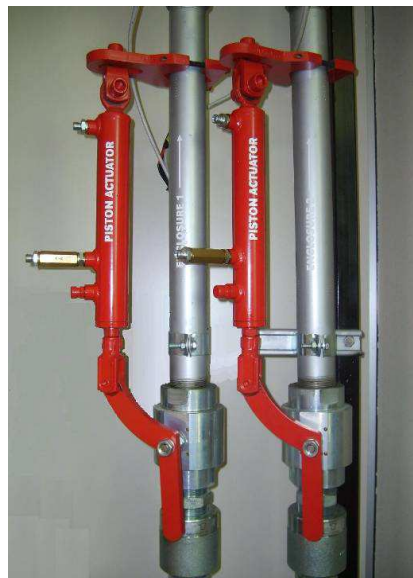
Fig.4.4 Pneumatic actuator pistons
