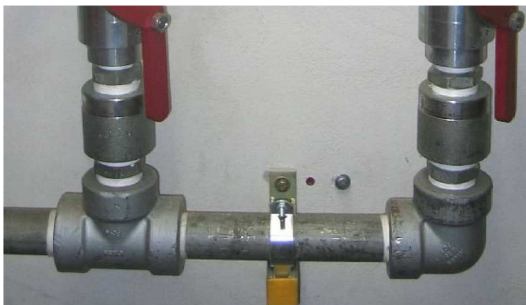
Fig. 4.2 Pressure reducing devices and nipples upstream of the directional valves assemblies
