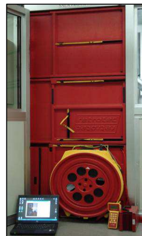
Fig. 5.1 Equipment for Door Fan Integrity Test
