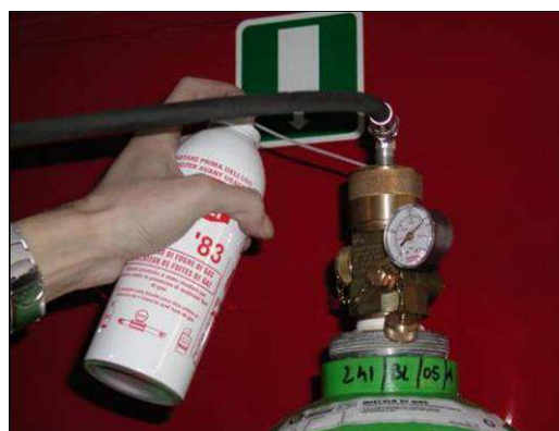
Fig. 5.5 Pneumatic circuit check (step 4, leak detection)
