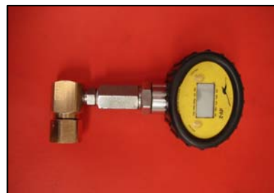
Fig. 3.2 Digital pressure gauge with swivel nut Bettati Mod dV-2
