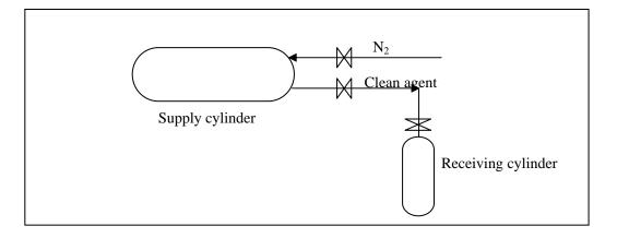
Put the supply cylinder on the higher site and let the receiving cylinder vacuum, then connect two cylinders. The gravity will let clean agent into the receiving cylinder.
