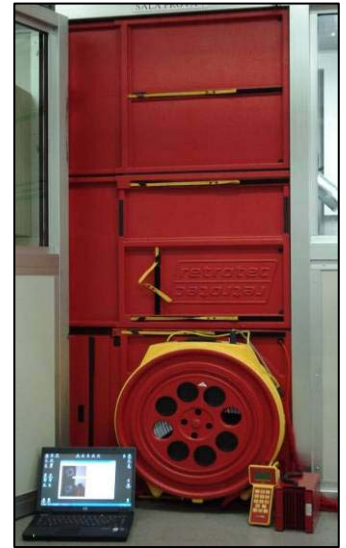
Figure 5.1 Equipments for door fan integrity test
