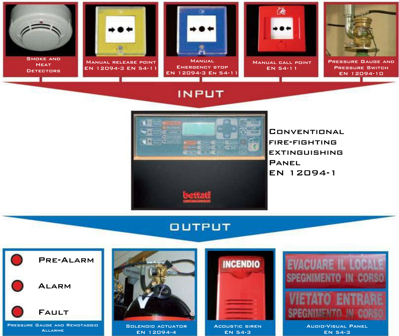
Fig.1.2 List of components of the detection system
